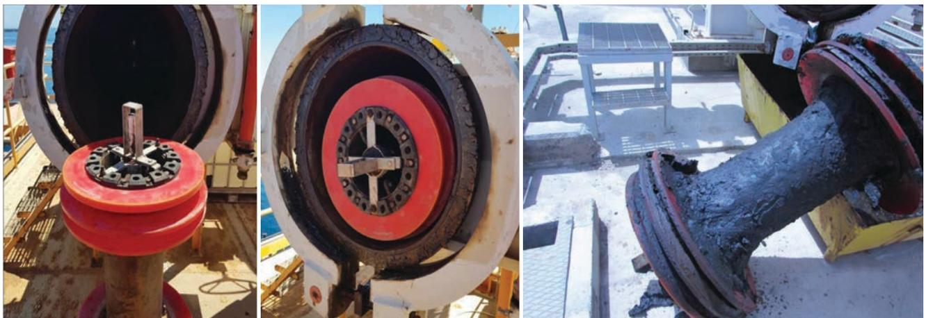
Figure 6: A look at the bidirectional polyurethane disc before and after pigging operations. Comparing the retrieved amounts of solids with the total length of the line shows that the intensity of the solids' distribution along the line is insignificant and unlikely to cause problems, validating the new flow assurance regime.
