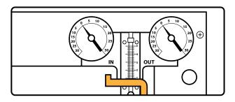
5. When a sample is ready to be collected, open the control handle until it "locks" into place. This closes off the flow to the IsoTube® into which your sample is collected, and switches flow through the BYPASS.
