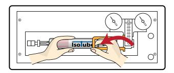
4. NOTE: Monitoring flow rates and pressures will aid in identifying any malfunctions. Both gauges should read approximately the same when the there is flow through either the IsoTube® or the bypass. A problem is indicated if there is no flow on the flow meter and/or if either gauge reads significantly different from the other.
