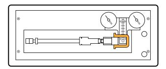
2. Insert the IsoTube® into the Manifold as shown. Some downward pressure must be applied to the "saddle" that locks the moveable chuck open when it is not in use
